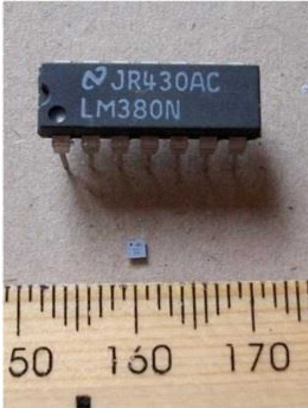
Figure 3 Left shows a previous and still current through hole power amplifier which can only deliver 2 watts of power into a loud speaker. Below that is the 3 watt Flip Chip amplifier of Figure 1 to show a size comparison.
